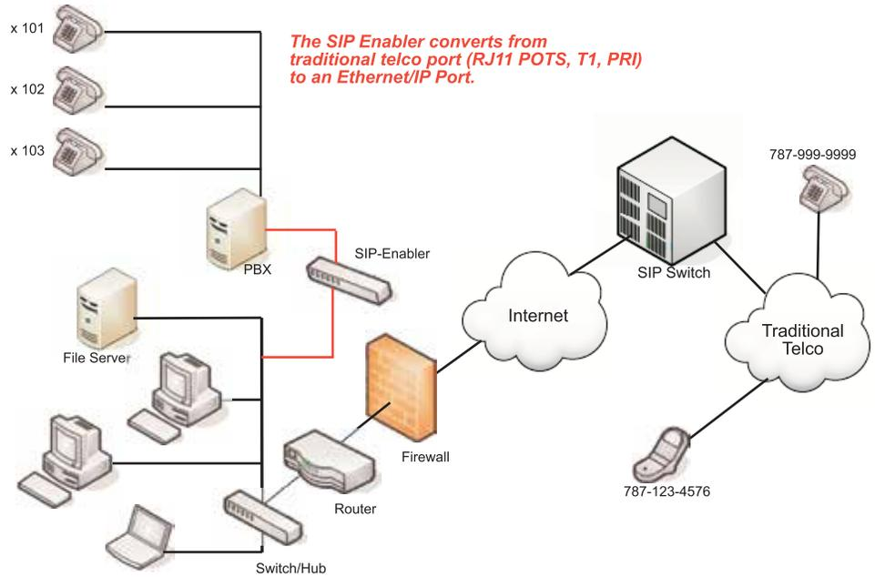
Sample SIP Trunking Network Diagram - SIP-Enabled PBX
